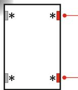
STAY GUARD ELITE SG025 on outer frame and sash for types of stay to include Egress/Easy Clean
